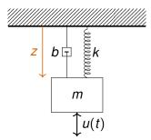
Model with external input u(t)  $\rightarrow$  Linear time invariant system X' = AX + Bu
